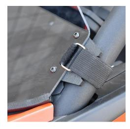
**Initial Assembly**. Use the supplied bolts and nuts to attach the plastic plates to the BACK of the windshield as pictured. Tighten the hardware so it is snug. (NO NEED TO TIGHTEN VERY TIGHT)
