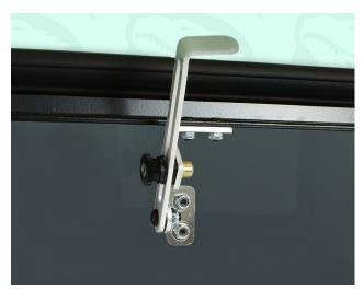
**STEP ONE –** Install both handle assemblies. Bolt the flap mount to the plastic flap using two  $10-24 \times 0.5$ " bolts. Attach the bracket with threaded insert to the bottom side of the bend on the windshield frame using two more  $10-24 \times 0.5$ " bolts and 10-24 lock nuts. Tighten bolts and loosen thumb screw to test if flap mechanism moves properly. Adjust the placement of the bracket with insert if the flap doesn't work.
