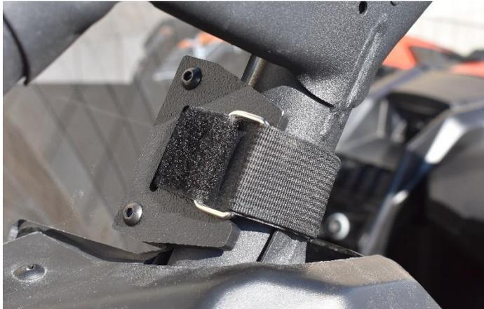
**Initial Assembly.** Use the supplied bolts and nuts to attach the plastic plates to the BACK of the window as shown in the picture above. To tell the front from the back look at the two bends near the top corners. The corners bend forward to follow the shape of the cage. Tighten hardware snug. Over tightening can cause damage to windshield.
