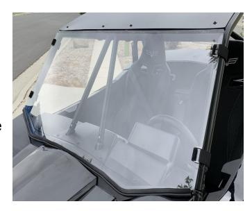
**Step 2:** Install straps with the fuzzy sides facing toward the center of windshield and the metal loop on the front side of the windshield.
