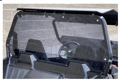
**Step 1:** Pull back protective film along edges on both sides of window. Install rubber edge trim along bottom edge of windshield for protection during install and use. This can be difficult. Rocking the trim back and forth while applying helps it go on easier. Cut excess trim with scissors or snips.
