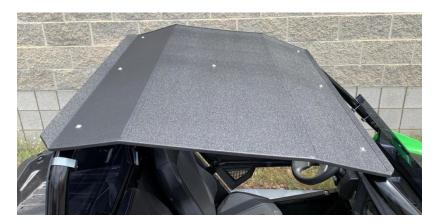
**Step 1:** Cut the edge trim in two equal pieces and install along the edges of roof for protection during install and use. This can be difficult. Rocking the trim back and forth while applying helps it go on easier. Cut excess trim with scissors or snips.
