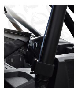
**STEP FOUR –** To completely wrap the velcro on the bottom straps you will need to place a sheet a paper, such as the instructions, in between the strap and push the end into place. Once the strap is in position pull the paper instructions out while holding the strap in place and it will let the velcro hook together. Repeat the process for both bottom straps. Once the top two straps are wrapped onto the cage the installation is complete.
