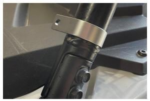
STEP 3. Place windshield on machine and loosely fasten in place using the .75" long bolts (with washer and lock washer) on the top mounts. Use the long 2.5" bolts with lock washer and flat washers to attach the bottom of the windshield by inserting the bolts through the windshield and billet clamp.
