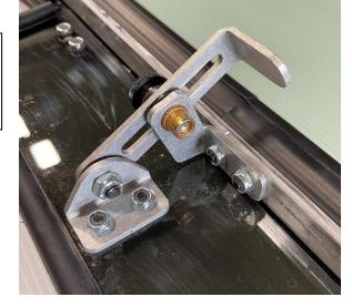
Place the two billet clamps as shown with the threaded hump on the back of the bar.
