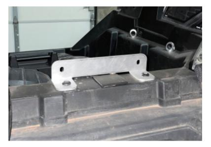
**STEP TWO –** Remove the film from both sides of the windshield. Install the windshield in place from inside the machine. Bolt the windshield to the mounting bracket using the provided bolts, nuts, and washers. Use a washer on both sides of the bolts. Insert the straps into each hole and tighten making sure to keep the windshield centered.
