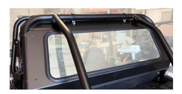
**Step 1:** Install rubber trim in designated locations. The long 47" Trim goes on the bottom edge of the metal frame. The 11" lengths go on the top corners of the metal frame. The 14.5" lengths go on the two notches on the plastic panel. (where harnesses may be attached to the cross bar)
