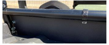
**Step 3:** Install glass windshield on outside of frame. Clip the clamps on approximate positions and lift windshield into place, (this is much easier with two people). Use remaining bolts, washers, and locknuts to secure in place as shown below.
