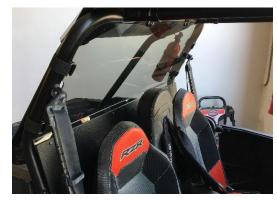
You can attach the lower panel before OR after installing the main window. It is easier to get the window in place if you install it before bolting on the lower panel. If you have harnesses already installed then you will want to bolt on the lower panel after you install the main window so you can place it around the harnesses.
