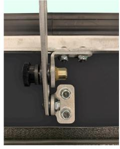
**STEP ONE** – Using the Handle Assembly bolt the Flap Mount on the inside of the polycarbonate as seen in the picture using 2 10-24 bolts and lock nuts. Tighten bolts. Mount the bracket with threaded insert on the right two holes of bottom brace using the other two 10-24 bolts and nuts.
