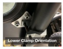
**STEP TWO** – Place the billet clamps on the frame with the clamp orientation shown in the picture. The flat face of the clamp should face forward and the clamp opening pointed towards the center of the machine. Use a 2.5" bolt with a washer to secure windshield to clamps. Adjust windshield to desired location and then tighten all the bolts.
