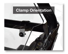
**STEP ONE** - Put the clamps on the roll cage in the approximate locations to line up with the holes in the window.
