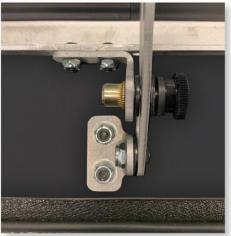
picture. The flat face of the clamp should face forward and the clamp opening pointed towards the center of the machine. Use a 2.5" bolt with a lock washer and a flat washer to secure windshield to clamps. Adjust windshield to desired location and then tighten all the bolts. **Do not over-tighten** the bolts causing the frame to distort it could cause the glass to break during a ride.
