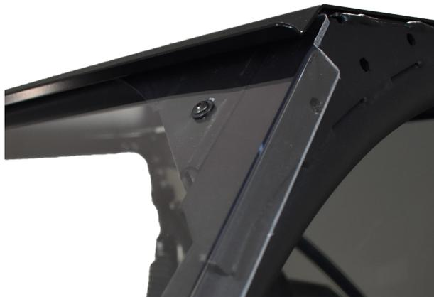
**STEP ONE** – Remove film and carefully place the bulb trim onto the bottom of the windshield. Place the windshield on the frame lining up the holes in the cage and windshield.
