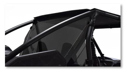
**STEP TWO** – While standing in the bed of the KRX put one corner of the window into place and squeeze the plastic together to get the other side into place. It rests towards the back of the machine, behind the brackets, where the cage meets the plastics.
