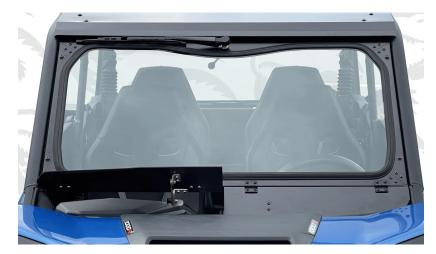
**Step One:** Remove any roof on the machine and replace after completing all the steps.
