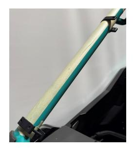
PRO R4 Optional Step. Because the regular top two mounting points are not used, you can plug them by installing the  $\frac{1}{2}$ " bolts with a lock washer, flat washer, oversized nylon washer, and lock nut.
