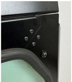
PRO R4 Step 6. Follow regular step 6 but make sure the top two holes in extension plate line up with the two front roof mount holes. If you don't have a roof, use the two 1" long bolts with washers and lock nut to attach the top of the windshield to the cage.
