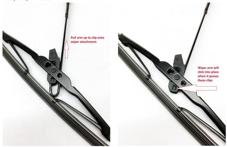
Step 2. Install wiper onto windshield as shown in pictures below. Install washers in same order on each side of frame.
